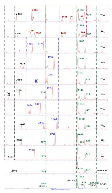
**Figure 2:** B3LYP/6-311++ $G^{**}$  calculated gas phase IR spectrum of the POSS-H<sup>+</sup>@W<sub>n</sub> (n=1-4) clusters. The three component bands (**A**) (black), (**B**) (blue) and (**C**) (brown) correspond to free water O-H stretching, to Eigen core to water stretching and to Zundel core proton oscillation, respectively.
