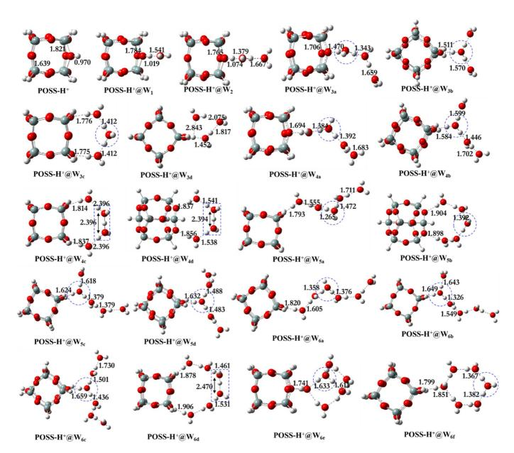
**Figure 1:** B3LYP/6-311++G\*\* optimized geometries of protonated polyhedral oligomeric silsesquioxane water clusters (POSS-H<sup>+</sup>@W<sub>n</sub>; where n = 1 - 6). Distances are in Å. The dashed blue circle and rectangle highlights the formation of H<sub>3</sub>O<sup>+</sup> and H<sub>5</sub>O<sub>2</sub><sup>+</sup> cations, respectively.
