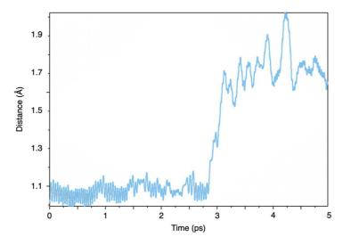
**Figure 3:** O\*-H<sup>+</sup> distance as a function of time during a 100 K AIMD simulation, where O\* is the oxygen atom of the POSS originally bonded to the excess proton in POSS-H<sup>+</sup>.
