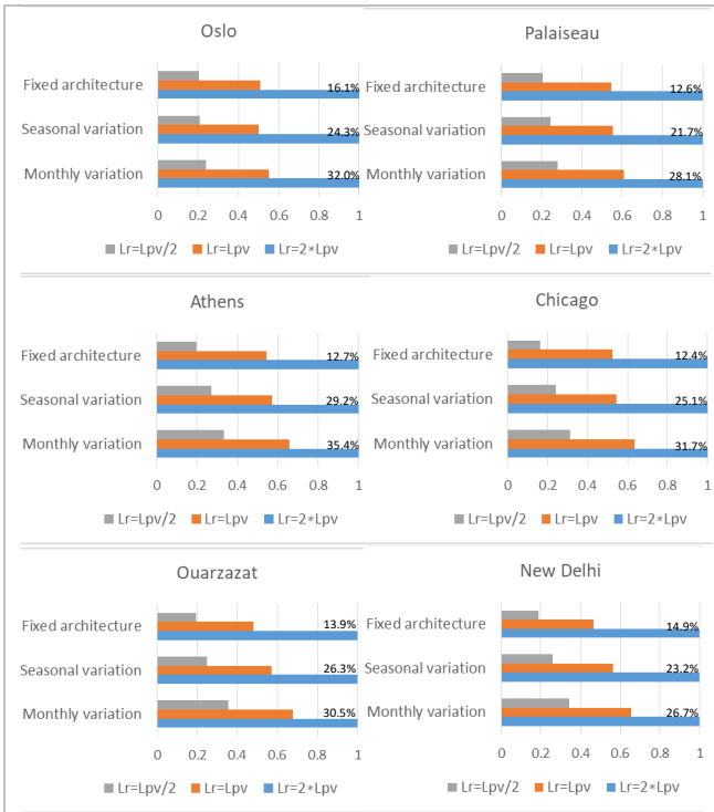
Fig. 5. Gain comparison according to the reflector's length
