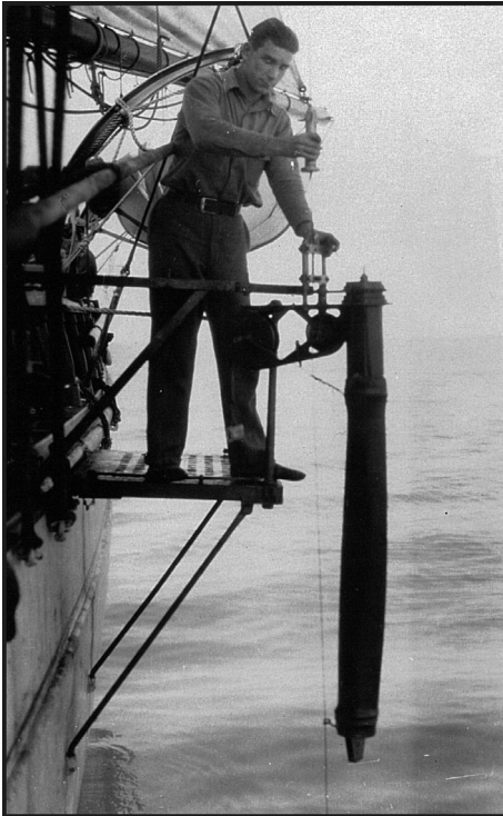
FIG. 4. Seiwell working the “plankton catcher” on the Carnegie . The Pettersson “Plankton Catcher” was installed on the Carnegie when the vessel was in Hamburg. It was designed to provide quantitative samples collected from a known volume of water (Pettersson 1928). In practice, it proved difficult to use (Paul 1932) and mainly provided qualitative samples. Image from Paul’s (1932) The Last Cruise of the Carnegie .
