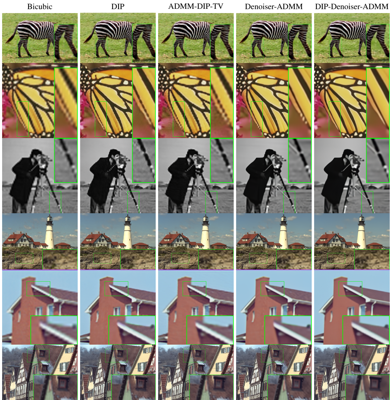
Fig. 3: Results obtained for the super-resolution application with magnifying factor of 4. The low resolution input image is generated using a Gaussian filtering kernel of standard deviation \sigma_f = 0.5 followed by a downsampling of 4.
