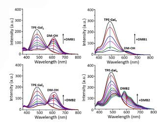
Figure 5. Fluorescence changes of TPE-Gal<sub>2</sub> (20  $\mu$ M) or TPE-Gal<sub>4</sub> (20  $\mu$ M) in PBS solution (pH 7.4, 0.01 m,  $\lambda_{ex}$ =320 nm) at 25 °C premixed with excess peroxynitrite (100  $\mu$ M), followed by addition of DMB1 (0–30  $\mu$ M) and DMB2 (0–50  $\mu$ M).
