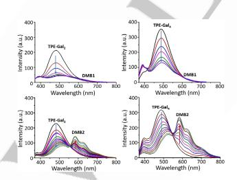
**Figure 4.** Fluorescence changes of **TPE-Gal**<sub>2</sub> (20 μM) or **TPE-Gal**<sub>4</sub> (20 μM) in PBS solution (pH 7.4, 0.01 M,  $\lambda_{ex}$  = 320 nm) at 25 °C with addition of **DMB1** (0–30 μM) and **DMB2** (0–80 μM).
