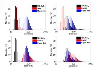
**Figure 2.** Aggregate size variation of DM probes, TPE-based glycoclusters and their glyco-dots after self-assembly obtained by DLS.
