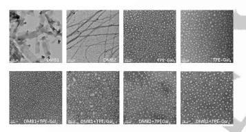
Figure 3. Aggregation of DM probes, TPE-based glycoclusters and their glyco-dots after self-assembly obtained by TEM.
