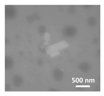
Figure 3. MEB-STEM image of Ni NHC-picolyl nanoparticles.
