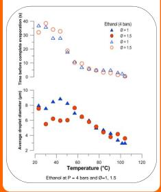
2. Pressure effect on droplets diameter & evaporation Increasing pressure reduces the vaporization time and produces a higher rate of vaporization, especially for small values of initial temperature.
