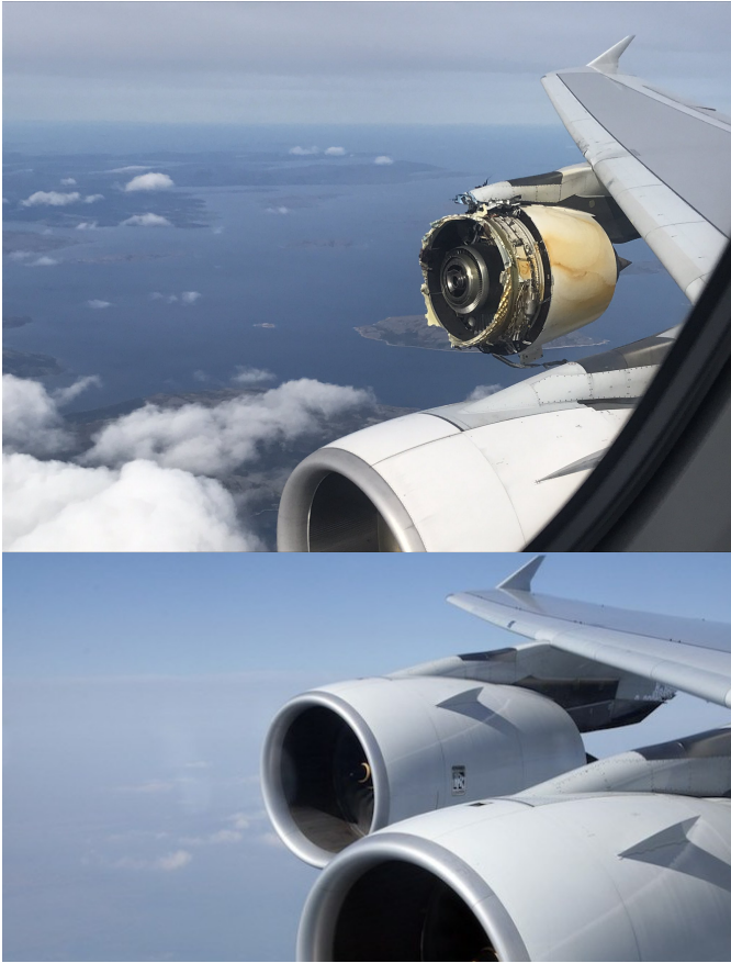
Fig. 1. F-HPJE engine #4 after unconfined failure (top) and image of a similar engine showing the missing fan assembly part (bottom).
