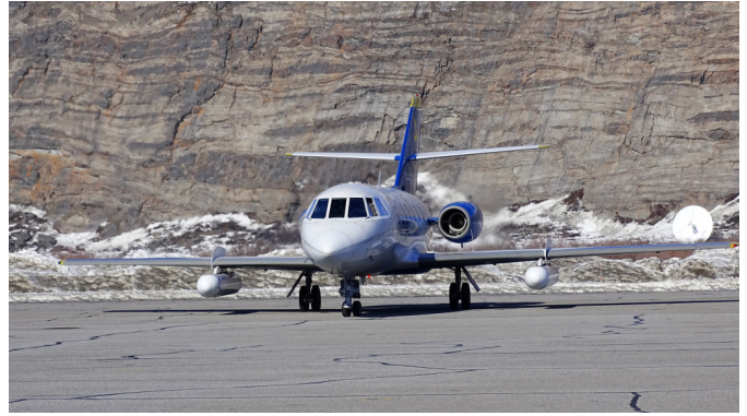
Fig. 3. ONERA SAR system “RAMSES” in the configuration used in Greenland. Pod under left wing (here on the right) contains the UHF sensor. Pod under the right wing (here on the left) contains the X-band sensor fore and the L band sensor aft. X-band sensor looks to the right (starboard) while both L & UHF band sensors look to the left (port).
