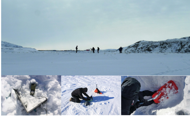
Fig. 4. Target setup: Calibrating corner reflector set in Kangerlussuaq (top). Corner reflector during burial (bottom left), Luneburg sphere half buried (bottom centre) and ice lens emulation during fabrication (bottom right).
