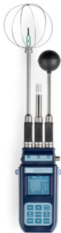
Figure 4. Thermal microclimate station.
