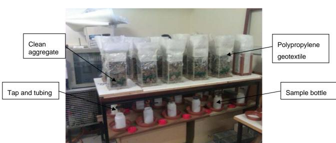
Figure 2 Experimental set up
