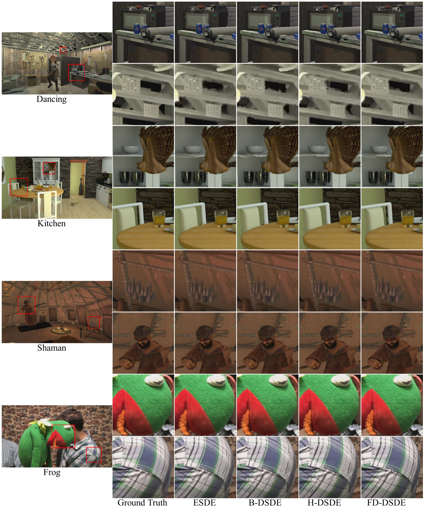
Fig. 9: Ground-truth and synthesized views with the proposed methods, for four sequences: Dancing, Kitchen, Shaman and Frog. FD-DSDE outperforms all other solutions visually.
