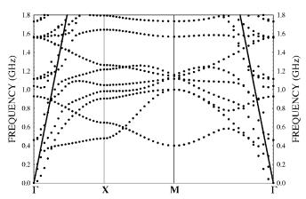
FIG. 5. Elastic band structures for the air/PZT phononic crystal plate of thickness h=a deposited onto a silicon substrate of thickness d=2h=2a. The thick solid lines represent the dispersion curves of the slower elastic waves propagating in an infinite, homogeneous medium composed of silicon, i.e., the waves of transverse polarization.
