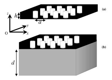
FIG. 1. (a) Freestanding phononic crystal plate of thickness h and (b) phononic crystal plate of thickness h deposited onto a homogeneous substrate of thickness d. The basic phononic crystal is composed of a square array of parallel cylindrical air inclusions (holes) of radius R drilled in a piezoelectric matrix. The lattice parameter is a. The cylindrical air inclusions are assumed parallel to the z axis of the Cartesian coordinates system (O, x, y, z).
