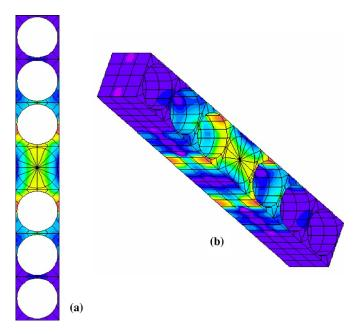
FIG. 4. (Color online) Maps of the modulus of the elastic displacement field for the waveguide mode with f=1.221 GHz and a wave vector of modulus 3.468  $\mu$ m<sup>-1</sup>; (a) top view and (b) three-quarter view. The red color corresponds to the maximum displacement, whereas the blue color corresponds to the minimum.
