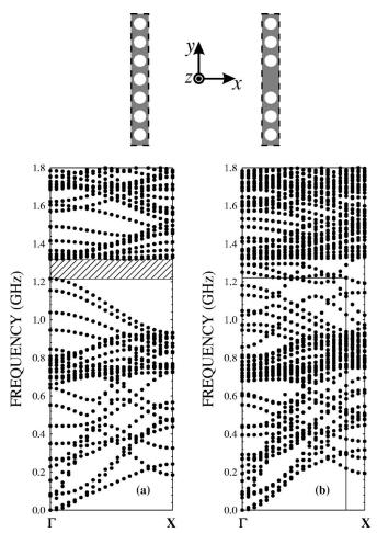
FIG. 3. Band structure along the  $\Gamma X$  direction calculated with a supercell containing  $1\times 7$  unit cell, for (a) the perfect phononic crystal plate and (b) the phononic crystal plate containing a waveguide formed by filling the hole in the fourth unit cell. The inset depicts the  $1\times 7$  supercell considered in each case. The two straight lines indicate the location of the guided mode analyzed in Fig. 4.
