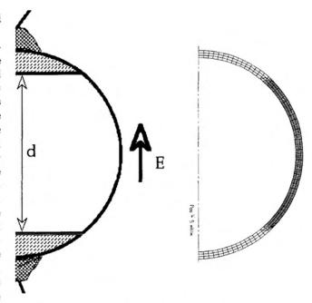
Fig. 3. Polarized region of a top-to-bottom poled sphere.
