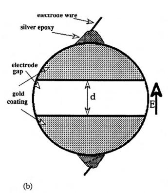
Fig. 1. Poling configurations: (a) radial poling configuration, (b) top-to-bottom poling configuration.
