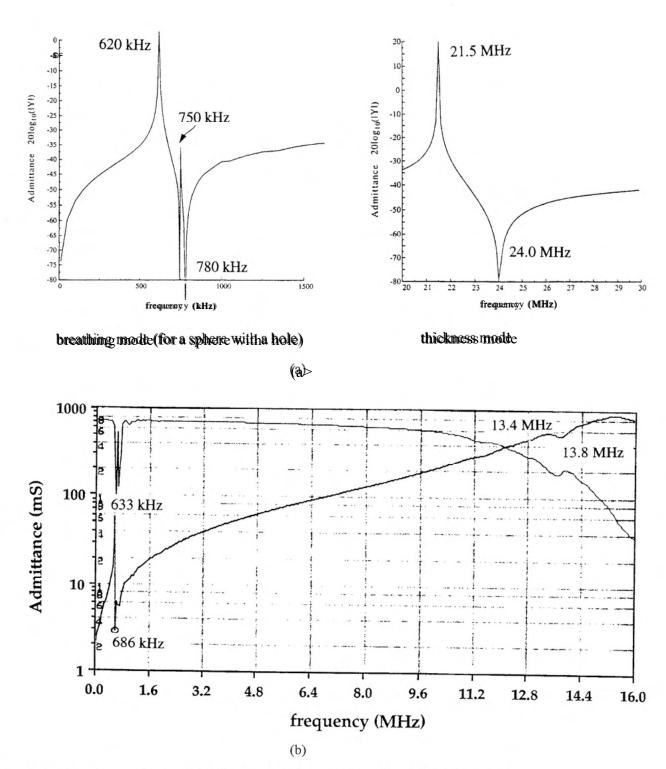
Fig. 22. Admittance speptratra of a radially poleted PZT hollow sphere transducturer: (ia) calculated, (b) observed.
