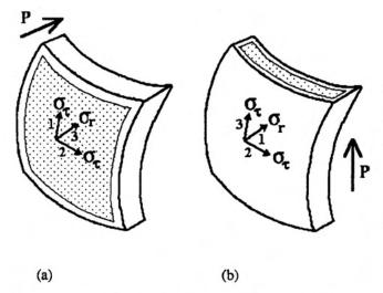
Fig. 8. Transformation of an applied hydrostatic pressure into radial and transgential stresses: (a) radial poling case, (b) top-to-bottom poling case.
