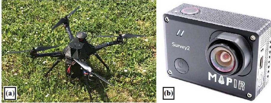
Figure 3: The acquisition equipment used in this study. The quadcopter UAV drone (a) and the high-resolution Survey2 sensor (b).
