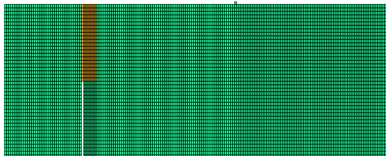
Figure 21: Macroscale mesh for mix-mode failure test
