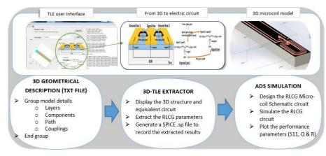
Fig. 1. Block diagrams of the simulation methodology: TLE user interface to 3D micro-coil model
