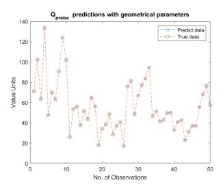
Fig. 3. The microprobe Q factor prediction and the true value parameters, working frequency and materials properties. As it is shown, our artificial intelligence algorithms (ANN) were validated to predict well (RMSE = 0.0316 Test dataset), the Q - factor of the microprobe even for a dataset of 6528 samples, which correspond to 99.8% for accuracy of the model prediction in term of to the Test performance.
