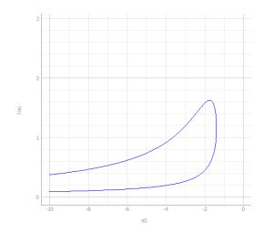
Fig. 1. Admissibility plot for a second-order retarded system with  $a_0=1,\ a_1=1,\ \tau_{\rm max}=3,\ {\rm and}\ s_{0,{\rm min}}=-10.$
