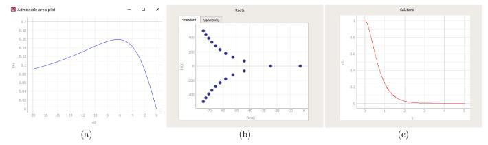
Fig. 2. Example of the usage of P3 $\delta$  in the "Control-oriented MID" mode for the delay-differential equation (3) with  $\omega = 2\pi$ . (a) Admissible region. (b) Roots of the characteristic quasipolynomial. (b) Numerical simulation of a solution with initial condition x(t) = 1 for  $t \leq 0$ .
