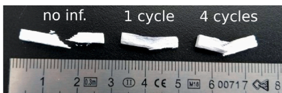
Fig. 5. Samples after mechanical testing. Porous ceramic (left) and composite after 1 (middle) and 4 (right) infiltration cycles. The porous composites are still holding as one piece after testing. The samples are from the tests reported in Fig. 4. © (2020) J. Seuba et al. (10.6084/m9.figshare.15022263) CC BY 4.0 license https://creativecommons.org/licenses/by/4.0/ .
