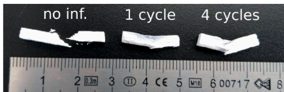
Fig. 5. Samples after mechanical testing. Porous ceramic (left) and composite after 1 (middle) and 4 (right) infiltration cycles. The porous composites are still holding as one piece after testing. The samples are from the tests reported in Fig. 4. © (2020) J. Seuba et al. (10.6084/m9.figshare.15022263) CC BY 4.0 license https://creativecommons.org/licenses/by/4.0/ .
