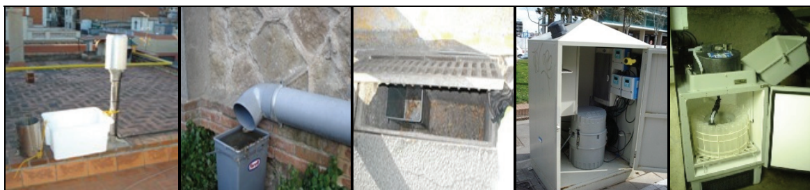
Figure 2: Some of the sampling devices used in the study (left to right): First to third: Accumulative sampler located on roof next to rain gauge (pure urban rainwater); on roof drainage (roof runoff point) and at sewer inlet (surface runoff point). Fourth and fifth: Automatic samplers at sewers and storm tank.
