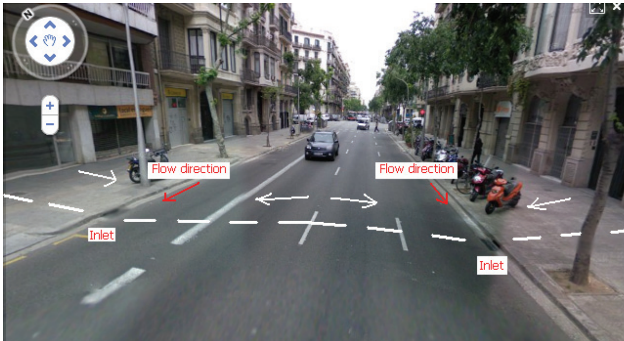
Figure 3: Representation of an urban subcatchment composed by 4 planes discharging to uniform triangular gutters. In this case the subcatchment hydrological limits are represented by the section where inlets are located
