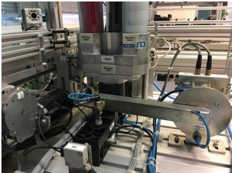
Figure 2. MAGASIN DE BOUCHONS ET VERIN ROTATIF
