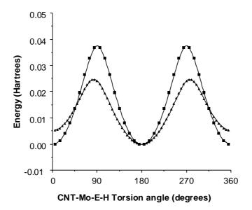
Figure 3. Plot of the energy of  $CpMo(EH_n)(PH_3)_2$  (S=0) vs. the CNT-Mo-E-H dihedral angle. All other geometrical parameters are those of the optimized geometry. Squares: E = P, n = 2; triangles: E = O, n = 1.
