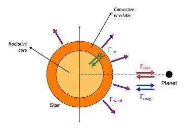
**Fig. 2.** Schematic view of the system and its interactions (adapted from Benbakoura et al. 2019). The radiative core (in yellow) and the convective envelope (in orange) exchange angular momentum (green arrows). Stellar wind carries away angular momentum from the envelope and spins the star down (purple arrows). Stellar rotation and planetary orbit are coupled through tidal (red arrows) and magnetic effects (blue arrows).
