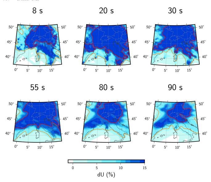
**Figure B1.** Results of flat tests. The input anomaly represents a velocity perturbation of 15 per cent at each gridpoint, that is a flat model. The recovered perturbations after regionalization are shown for periods 8, 20, 30, 55, 80 and 90 s. Red lines represent a velocity anomaly of 14 per cent, that is 90 per cent of the input perturbation. Orange lines represent an anomaly of 5 per cent, that is 30 per cent of the input model.
