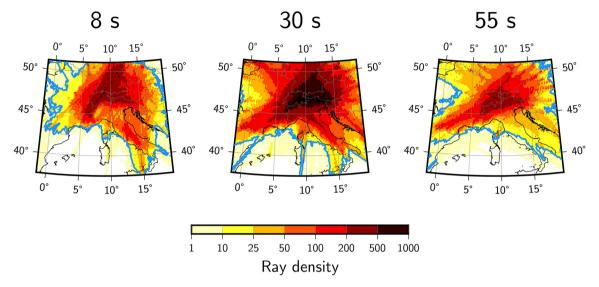
Figure A1. Ray density maps at periods 8, 30 and 55 s showing the number of paths crossing each  $0.15^{\circ} \times 0.15^{\circ}$  cell. The blue line delimits the area with ray density higher than 10.
