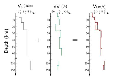
Figure 5. Illustration of the model parametrization: (left-hand graph) layered reference model  $V_0(z)$  that remains fixed during the inversion; (middle panel) model of velocity variations dV(z) defined by layers whose number, thickness, and velocity change dV are unknowns of the inversion; (right-hand graph) final model constructed by adding the perturbations to the background model.
