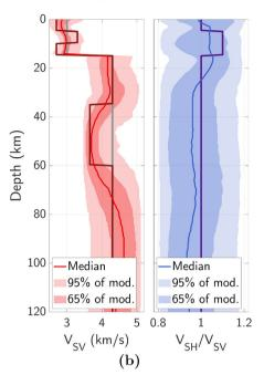
**Figure 7.** Synthetic tests where the same data produced by the true model are inverted with two different procedures. Left-hand panels: inversion used in this study, where each layer can either be isotropic or anisotropic. Right-hand panels: inversion where anisotropy is imposed as an unknown parameters at all depths. See legend of Fig. 6 for the meaning of the different lines and colours.
