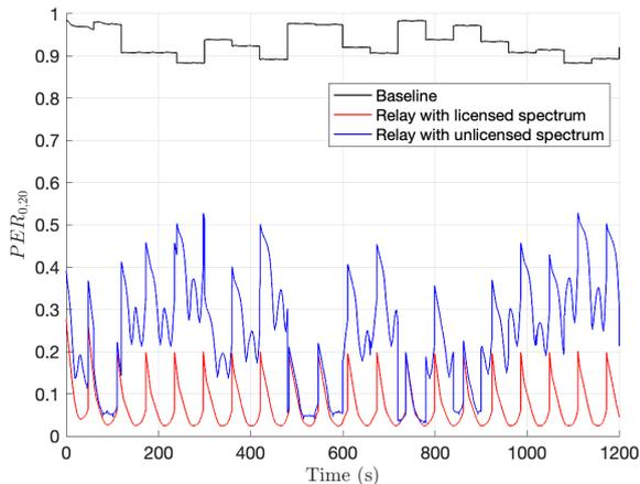
Fig. 5. PER for 20th vehicle for the different communication scenarios.
