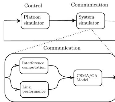
Fig. 4. System diagram with control and communication interaction.
