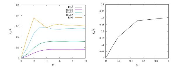
FIG. 2. Evolution of the ratio of turbulent potential to kinetic energy  $K_{\rho}/K$  in nondimensional time St (left) and dependence of this ratio on the Richardson number at St = 10 (right).
