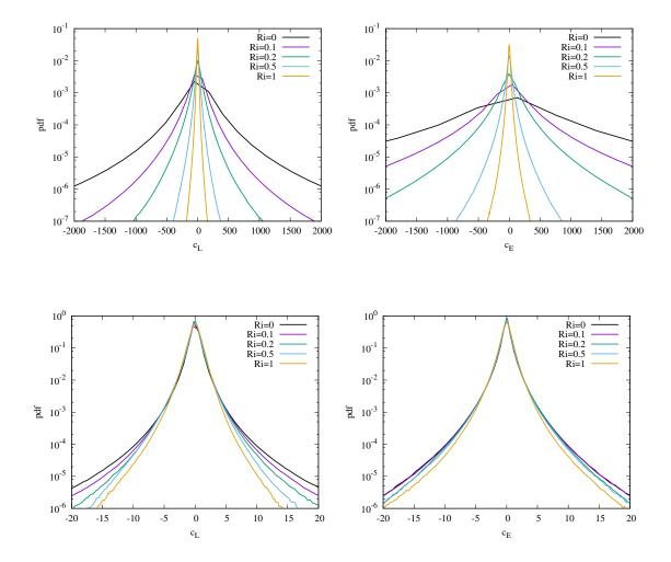
FIG. 11. Pdfs (top) and normalized pdfs (bottom) of Lagrangian time-rate of change of vorticity  $c_L$  (left) and Eulerian time-rate of change  $c_E$  (right) at nondimensional time St=10. Note that pdfs for the vector quantities are shown.
