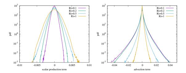
FIG. 10. Pdfs of the buoyancy (left) and advection (right) terms in the advection-diffusion equation for fluctuating density at nondimensional time St = 10.
