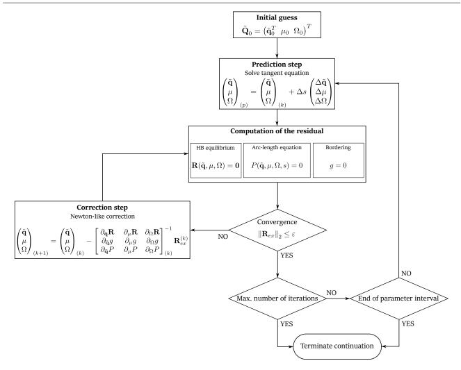
Fig. 4: Flow chart of the bifurcation tracking algorithm
