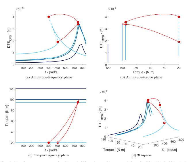
Fig. 13: Forced response curves and saddle-node bifurcation tracking curve. Coloured solid and dashed lines in the amplitude-frequency planes correspond to stable responses and unstable responses, respectively. Red circle markers ( $\bullet$ ) denote saddle-node bifurcations. The saddle-node tracking curve is represented as a red solid line (--).
