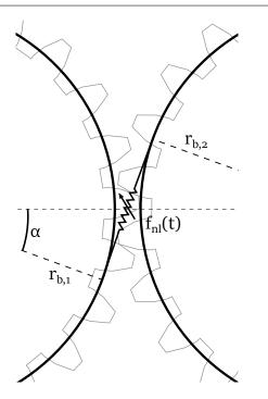
Fig. 5: Nonlinear gear model.
