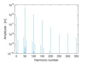
Fig. 12: Spectral content of the response on the upper branch of primary resonance at  $\Omega = 400$  rad/s showing negligible harmonics.
