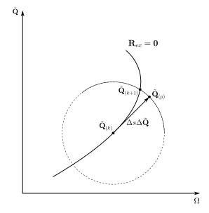
Fig. 2: Illustration of the arc-length continuation.
