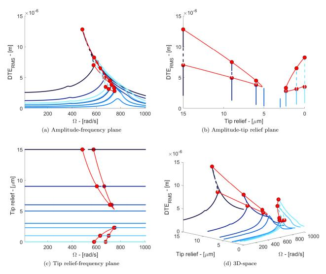
Fig. 14: Forced response curves and saddle-node bifurcation tracking curve. Coloured solid and dashed lines in the amplitude-frequency planes correspond to stable responses and unstable responses, respectively. Red circle markers
