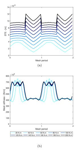
Fig. 7: Time evolution of the static transmission error and mesh stiffness computed by solving Eq. (38) and reconstructed with 6 harmonics for torque values ranging from 20 N·m (—) to 200 N·m (—)
