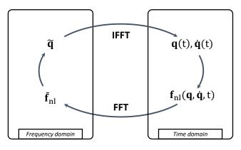
Fig. 1: Illustration of the implemented AFT procedure.
