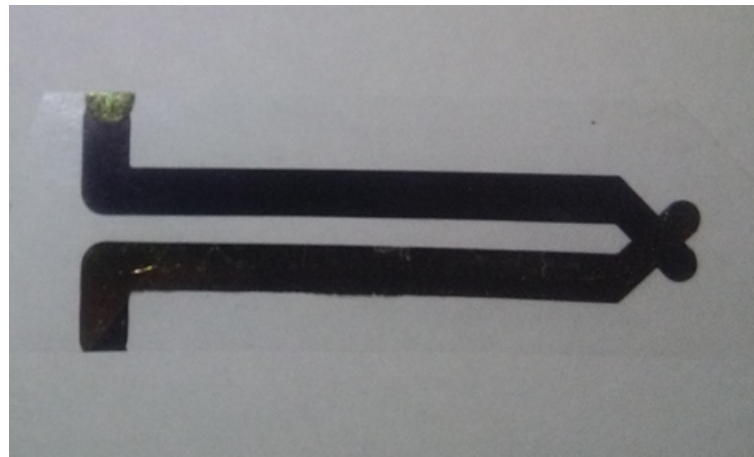
Figure 1. Bauer S25 PVDF bare shock gauge. Leads are on each side of the tape, sensing area is located at their facing portions.
