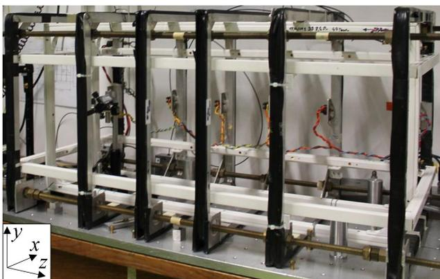
Figure C.1: View of the assembled set of magnetic field coils (see text).
