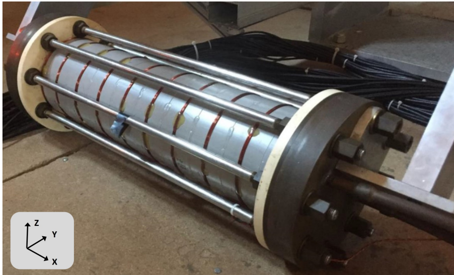
Figure 5: Hollow ferromagnetic cylinder filled by pressurized oil, with its degaussing windings.
