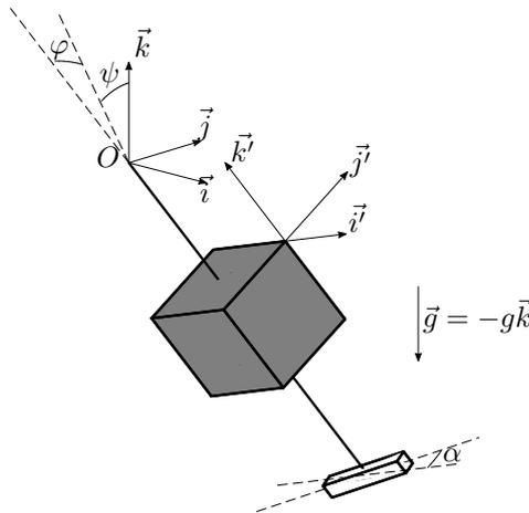
Figure 1: The main system: a two-degrees-of freedom pendulum under gravitational effects with  $\vec{g} = -g\vec{k}$ .
