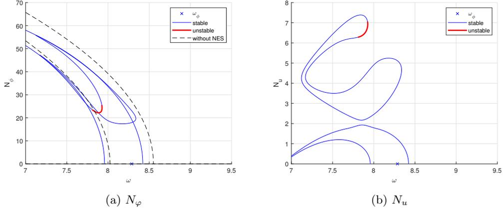
Figure 7: Equilibrium points of the system for a vertical excitation  $z_2 = 0.05$ .
