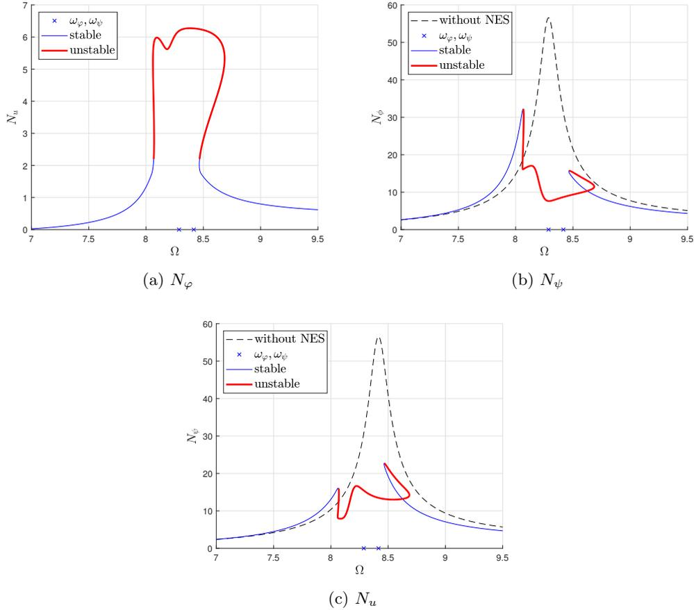
Figure 4: Equilibrium points of the system for a horizontal excitation  $x_1 = 17$  mm.
