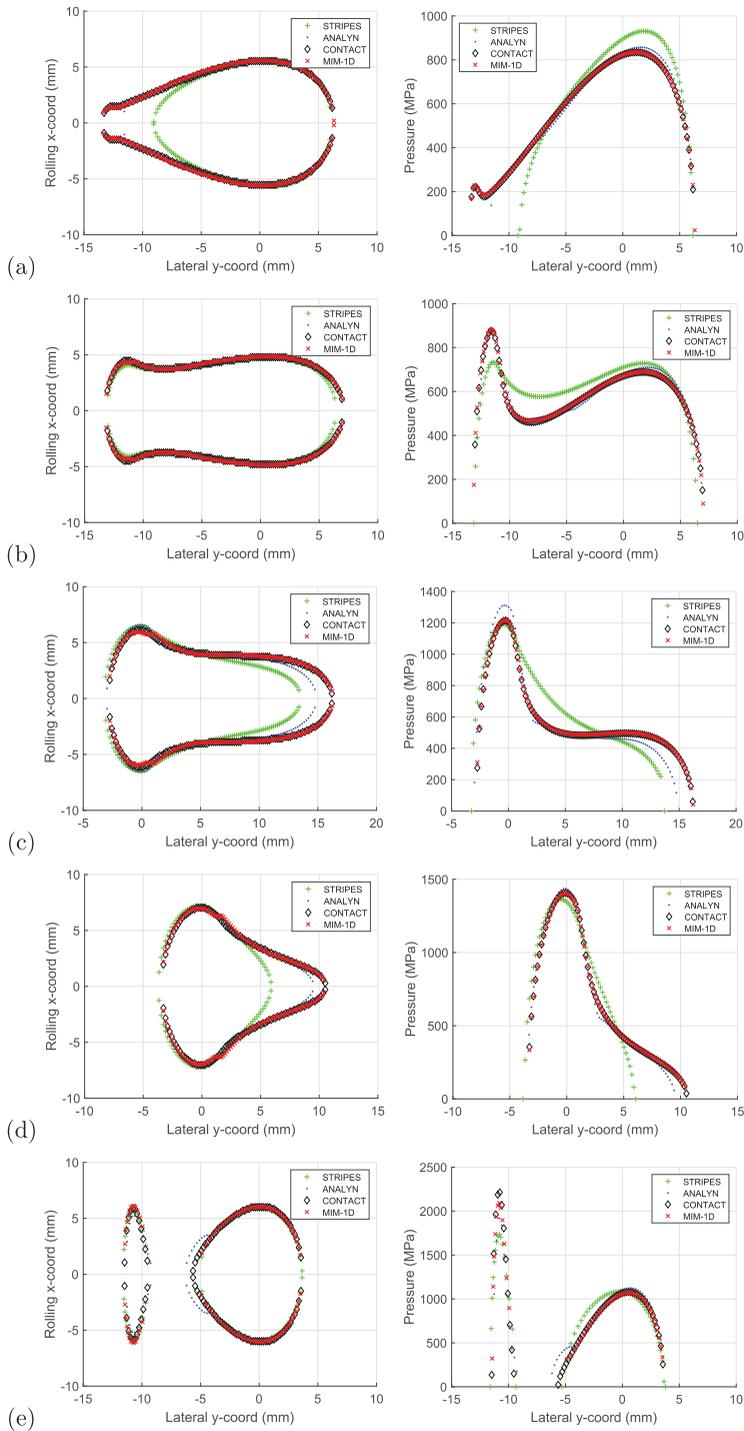
**Figure 8.** Contact patch (left), and the maximum pressure distribution  $p_0(y)$  (right) for wheel–rail contact cases (from top to bottom): (a)  $\Delta y = -1$  mm, (b)  $\Delta y = 0$  mm, (c)  $\Delta y = 1$  mm, (d)  $\Delta y = 2$  mm, and (e)  $\Delta y = 5$  mm.
