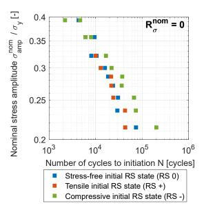
Figure 8: Experimental fatigue life under repeated tensile loadings for the three initial residual stress states
