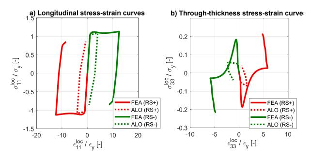
Figure 11: Stress-strain curves at the critical point during the introduction of residual stress in the (a) longitudinal and (b) through-thickness directions
