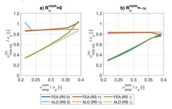
Figure 18: Predicted equivalent maximum stress for the three initial residual stress states at  $R_{\sigma}^{nom} = 0$  (a) and  $R_{\sigma}^{nom} = -\infty$  (b)
