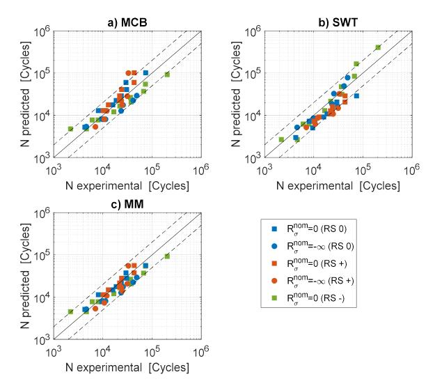
Figure 20 : Experimental vs. predicted fatigue life for the three initial residual stress states and the two load ratios with a) MCB, b) modified Morrow's and c) Smith-Watson-Topper criteria
