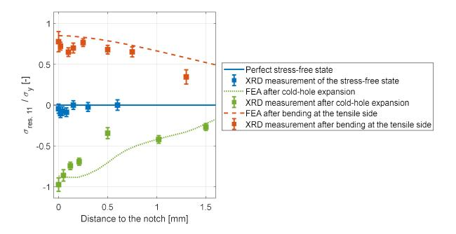
Figure 6: FEA predicted initial residual stress gradients compared to the IXRD corrected measurements 1.4 Fatigue testing of the notched specimens
