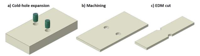
Figure 4: Principle of the cold-expansion process
