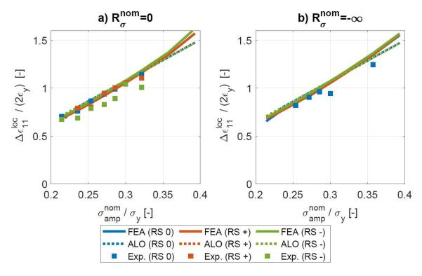
Figure 14: Longitudinal strain amplitudes for the three initial states at  $R_{\sigma}^{nom} = 0$  (a) and at  $R_{\sigma}^{nom} = -\infty$  (b)
