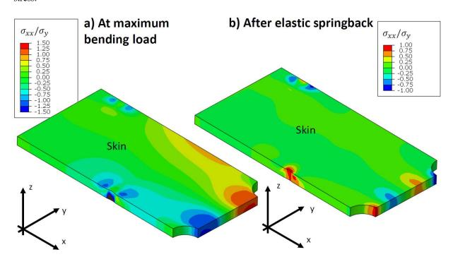
Figure 3: Bending simulation results at maximum bending load (a) and after elastic springback (b). Stress results are divided by the tensile yield stress
