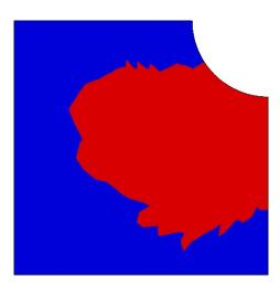
Figure 12: Yielding zone around the notch during bending for the introduction of residual stresses
