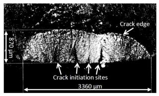
Figure 7: a) Evolution of ACPD signal for specimens under tensile or compressive repeated nominal loading and b) fracture surface obtained for a test stopped at a 0.02V variation criterion
