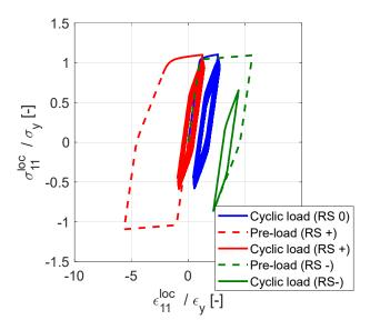
Figure 13: Introduction of residual stresses and cyclic loading for the three initial states at  $R_{\sigma}^{nom} = 0$  at a nominal stress amplitude of  $0.29\sigma_{\nu}$  predicted with the ALO method
