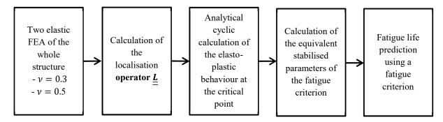
Figure 10: Fatigue life design methodology using the ALO method
