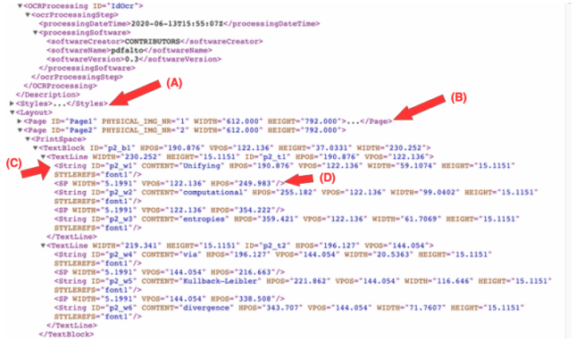
Figure 3: Result of the processing by pdfalto : (A) style block (information about fonts); (B) page block; (C) character string; (D) spacing information
