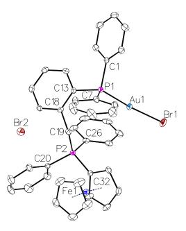
Figure 2: ORTEP view of complex le Au1-Br1: 2.4026(4); Au1-P1: 2.2373(9); P1-Au1-Br1: 172.73(2). Thermal ellipsoids are drawn at 50%
