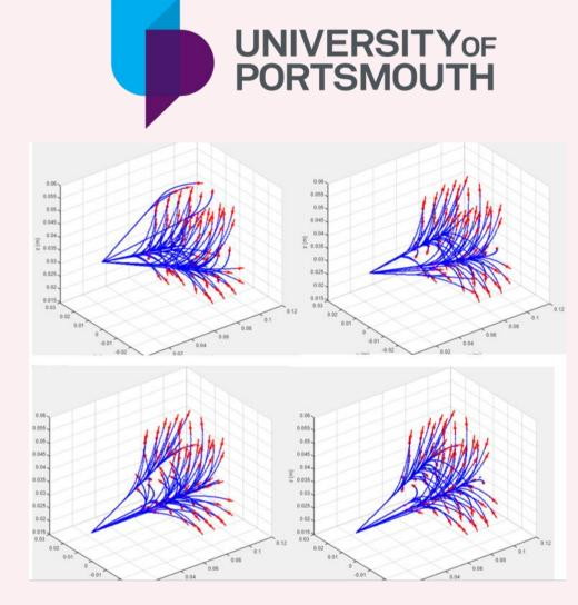
*Figure 5. Example image of* trajectory outcomes from CoBra software (seeds in red, needle paths in blue).
