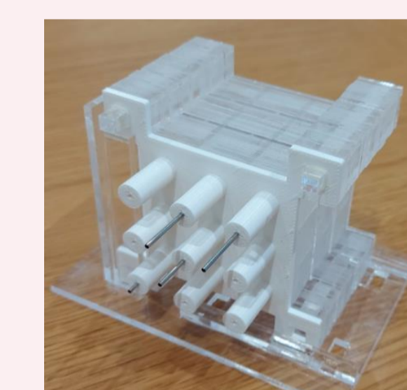
Figure 3. QA internal grid with needle guide (50x50x50mm).
