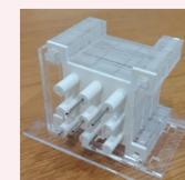
Figure 3. QA internal grid with needle guide (50x50x50mm).
