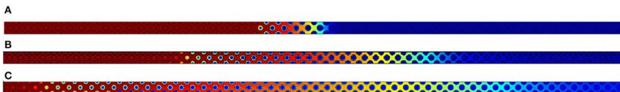
FIGURE 7 | Oxygen concentration fields obtained respectively for (A) Pe_{p,O_2} = 2.5 , (B) Pe_{p,O_2} = 10 and (C) Pe_{p,O_2} = 20 . Concentration varies from 0 in dark blue to its maximum value 1 in dark red.
