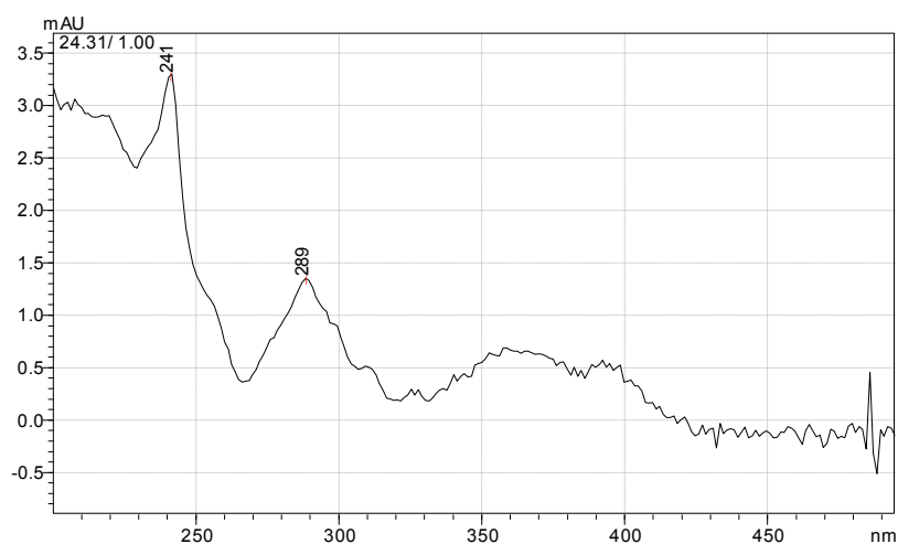
Figure S14. The fraction eluted from the solid-phase extraction column between 27.00-29.00 min was re-injected into the HPLC system. In this figure we can see UV spectrum of pyrene-3-carboxaldehyde eluted from the HPLC column at 24.31 min.
