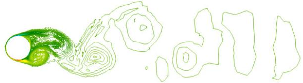
Figure 19: Instantaneous vorticity magnitude at the spanwise mid plane for a LES (Run 7).
