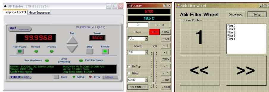
Figure 6: PISCO2: remote control of the Risley prisms (left panel), motorized focusing (central panel) and filter wheel selection (right panel).
