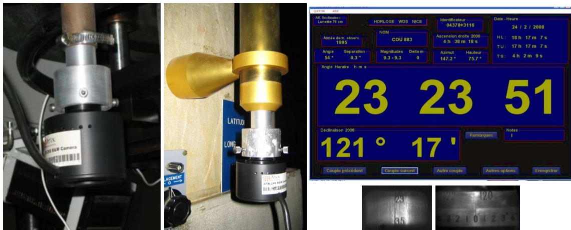
Figure 2: Webcams used for reading the hour angle (H.A.) and declination (Dec.) circles and thus allowing remote control of the L76 refractor. Left panel: H.A. webcam, central panel: Dec. webcam, upper right panel: Horloge program (from G. Morlet), lower right panel: webcam images of the H.A. and Dec. circles.
