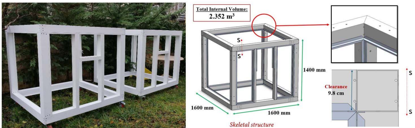
Figure 1 Skeletal structure of the modular prototypes.
