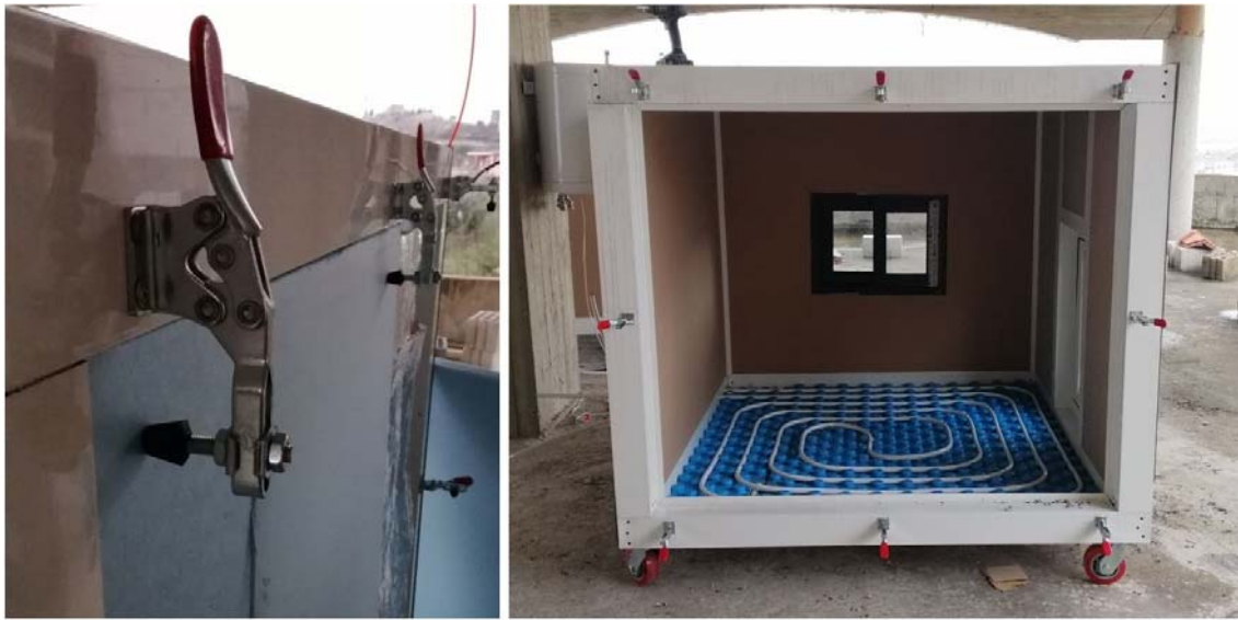
242 Figure 3 Hold down toggle clamps implemented in the west walls of the prototypes for facilitating assembling and 243 reassembling.
