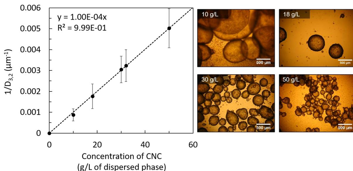
Figure 10: Left, Reverse drop diameter as a function of the amount of CNC-Br in the organic IPM phase for the SI-ATRP system. All the other parameters are kept constant: 25/75<sub>v/v</sub>, OEGMA 40 wt%, [OEGMA]/[CuBr<sub>2</sub>]/[TPMA]/[HOEBib] = 200/0.5/0.5/1. The linear variation highlights the limited coalescence phenomenon occurring in this concentration range. The error bars reflect the drops size distribution width. Right, optical microscopy observation of according emulsions.
