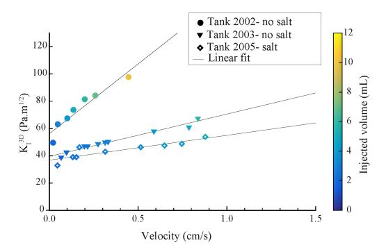
Figure 12: Stress intensity factor  $K_I^{3D}$  as a function of vertical velocity. 26 air injections for 3 different tanks (2002 and 2003 unsalted and 2005 salted) are represented. The stress intensity factor is estimated from the 3D theory (Eq. 14). For each tank, the limit of  $K_I$  when the vertical velocities tends to zero corresponds to the fracture toughness of the gelatin.
