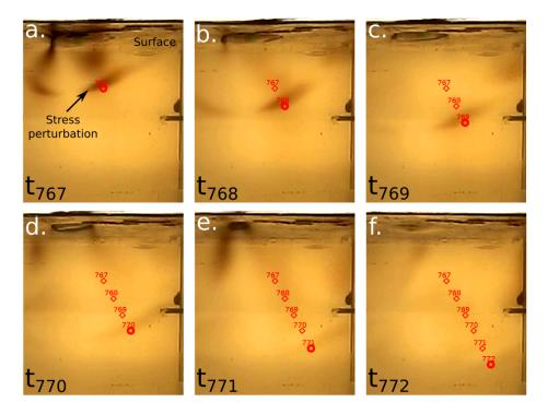
Figure 2: Shear wave velocity measurements with TRACKER. Panels (a to f) display screenshot of six successive images ( $t_{767}$  to  $t_{772}$ ) from the video records of tank 1910 showing shear wave propagation front after exciting the surface. Red dots indicate the manual picking of the propagation front position to compute the velocity. Note that the shear wave attenuates quickly and it becomes increasingly difficult to track it manually.
