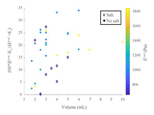
Figure 10: Relative difference between the Young's modulus estimated by air-filled crack length  $(E_{\alpha})$  and by surface loading  $(E^{load})$  for four tanks (2002, 2003, 2004 and 2005 as listed in Tab 1). Circles and diamonds represent injections inside unsalted gelatin and salted gelatin, respectively. Colors represent the Young's modulus  $(E=E^{load})$  of the tank estimated by surface loading.  $E_{\alpha}$  is computed with  $\alpha=0.25$  in Eq. 11.
