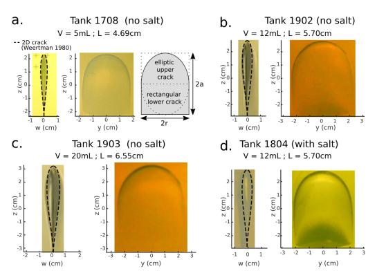
Figure 8: Panels (a), (b), (c) and (d) show crack shapes in cross section (left) and front (right) view of four experiments. Profile opening along cross sections is computed with Eq. 9 (dashed line). Panel (a) also shows a scheme of the theoretical shape of front view as a combination of an elliptic upper part which radius are r (half-width) and a (half-length) and a rectangular lower part which sides are 2r and a.
