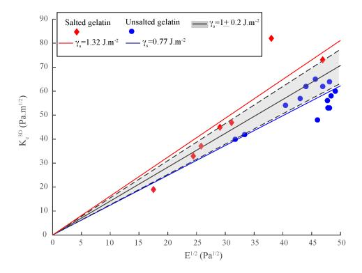
Figure 13: Relationship between the fracture toughness and the Young's modulus. Fracture toughness is estimated using the 3D approximation (Eq. 14). Linear fit, with uncertainties, corresponding to  $\gamma_s$  equal to  $1\pm0.2~\mathrm{Jm^{-2}}$  [33, 16] is represented by the black line, whereas fits obtained from the salted and unsalted tanks are represented, respectively, by red and blue lines.
