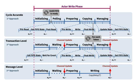
**Figure 4.** Simulation steps of the model of an actor write phase using two different communication models. cycle accurate [5] model at the top, message level [6] at the bottom and new transaction level model in the middle.
