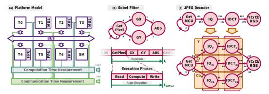
**Figure 2.** (a) Shows the architecture model of our evaluation platform (purple) and the measurement infrastructure (green) for characterization. (b) Shows details of the computation model on our Sobel-Filter Use-Case. (c) Shows our JPEG decoder Use-Case with and without considering data dependent behavior.
