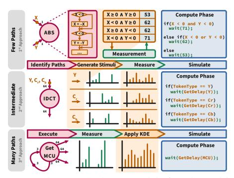
**Figure 3.** Modeling process with explicit execution path identification shown at Sobel-Filter example actor *GetPixel* (**top**), using Kernel Density Estimation shown at JPEG-Decoder example actor *GetMCU* (**bottom**) and a combination of both for actor *IDCT* (**middle**).
