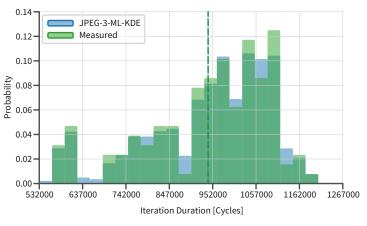
(d) JPEG Decoder on 3 Tiles (Realistic Mapping) using best communication and computation model.
