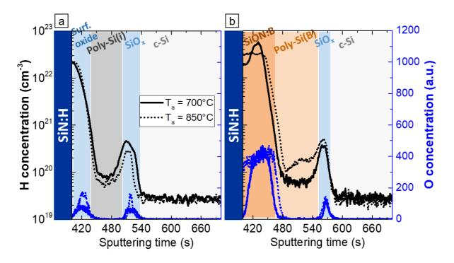
**Figure 7**. H and O concentration profiles (represented by black and blue lines, respectively) as measured by ToF-SIMS on samples featuring the poly-Si(i)/SiO<sub>x</sub> (a) and the poly-Si(B)/SiO<sub>x</sub> (b) contacts. Measurements were performed after SiN:H deposition on samples annealed at  $T_a = 700$  °C (solid curves) and 850 °C (dashed curves).
