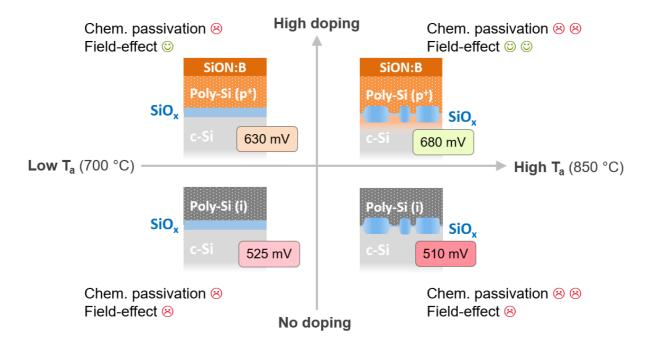
**Figure 8**. Schematic picture summarizing the respective effects of chemical and field-effect passivation of B-doped (top) and intrinsic (bottom) samples after the annealing step used for crystallization and doping of the poly-Si layer, as a function of the annealing temperature ( $T_a$ ). For the sake of simplicity, only the extreme  $T_a$  of the range investigated in this work are represented (i.e. 700 °C and 850 °C) with corresponding iV<sub>oc</sub> values.
