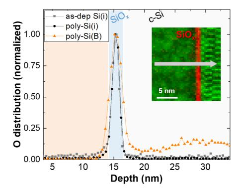
**Figure 5.** O distribution profiles assessed by EELS after deposition of the intrinsic Si layer (asdep Si(i)), after annealing at  $T_a = 800$  °C (poly-Si(i)) and after SiON:B deposition plus annealing at  $T_a = 800$  °C (poly-Si(B)). Each profile is an average of the profiles extracted from the respective EELS image along the direction perpendicular to the sample's surface (see arrow in the inset). The intensity of the O peaks was normalized to their maximum value.
