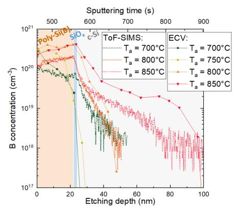
**Figure 6**. Active and total B concentration profiles measured by ECV and ToF-SIMS, respectively, on ex-situ doped poly-Si/SiO<sub>x</sub> contacts after annealing at various annealing temperatures T<sub>a</sub>. The etching depth on the bottom x-axis and the sputtering time on the top x-axis refer to the ECV and ToF-SIMS measurements, respectively. The SiON:B doping layer was not etched before ToF-SIMS analysis but is not represented in this graph.
