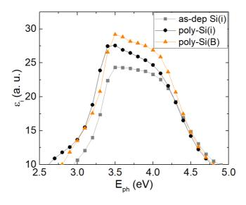
**Figure 4**. Imaginary part of the pseudo-dielectric function ( $\epsilon_i$ ) versus photon energy ( $E_{ph}$ ) obtained by spectroscopic ellipsometry (SE) measurement of the as-dep Si(i) layer after deposition, the poly-Si(i) layer after deposition and annealing at  $T_a = 800$  °C and the poly-Si(B) layer after deposition of the SiON:B doping layer on top of the as-dep Si(i) layer and annealing at  $T_a = 800$  °C.
