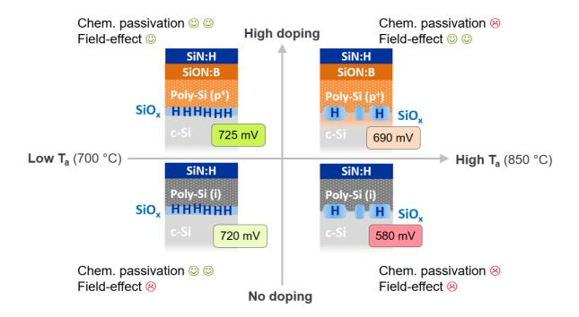
**Figure 9**. Schematic picture summarizing the respective effects of chemical and field-effect passivation of B-doped (top) and intrinsic (bottom) samples after subsequent hydrogenation and firing steps as a function of the annealing temperature (T<sub>a</sub>). For the sake of simplicity, only the
