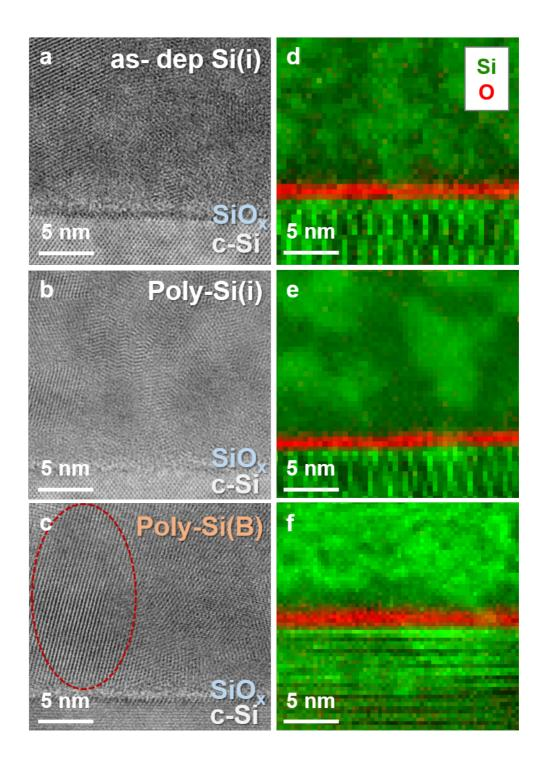
**Figure 3.** HR-STEM images of the as-dep Si(i) layer after deposition (a), the poly-Si(i) layer after deposition and annealing at  $T_a = 800$  °C (b) and the poly-Si(B) layer after deposition of the SiON:B doping layer on top of the as-dep Si(i) layer and annealing at  $T_a = 800$  °C (c). The respective EELS elemental maps of these samples (d) (e) and (f) are depicted beside the STEM images (we note that STEM images and EELS maps were not measured exactly in the same areas).
