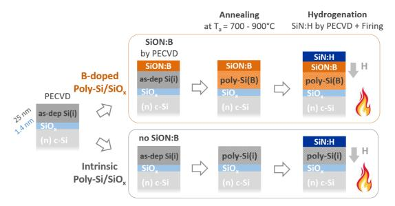
Figure 1. Schematic of the fabrication processes of B-doped and intrinsic poly-Si/SiO<sub>x</sub> contacts.
