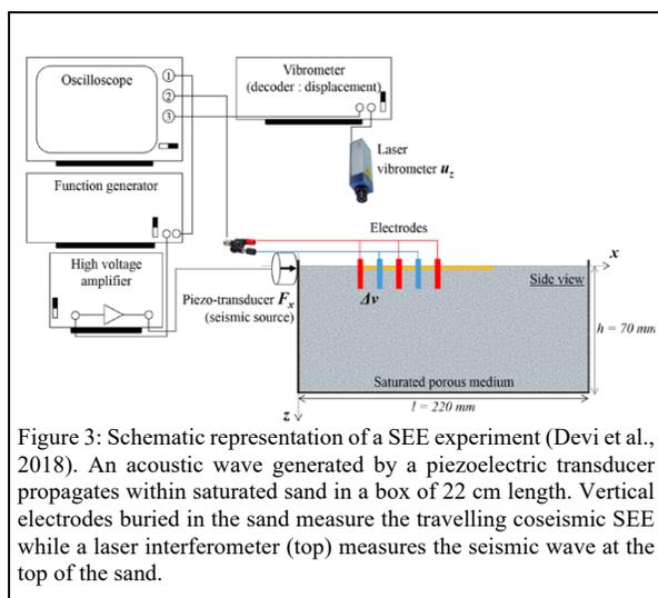
Figure 3: Schematic representation of a SEE experiment (Devi et al., 2018). An acoustic wave generated by a piezoelectric transducer propagates within saturated sand in a box of 22 cm length. Vertical electrodes buried in the sand measure the travelling coseismic SEE while a laser interferometer (top) measures the seismic wave at the top of the sand.
