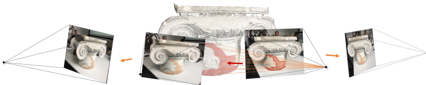
Fig. 4 - Aioli's approach for 2D/3D propagation of 2D regions, based on the spatialization of project resources.
