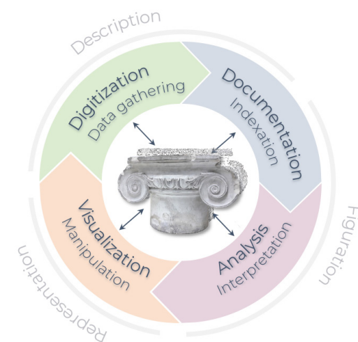
Fig. 3 - A methodological challenge: the union of the survey phases in a single moment facing the real object. The survey must be considered as a cycle whose different phases are centered on the study object, possibly through its 3D copy.
